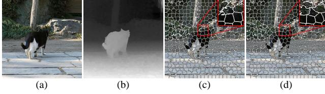
**Fig. 2.** Comparison of the primary SLIC and the extended SLIC for RGB-D image. (a) and (b) Color channel and depth channel of RGB-D image. (c) Super-pixels generated by the primary SLIC. (d) Super-pixels generated by the extended SLIC for RGB-D image.
