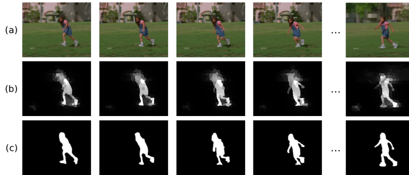
Fig. 1.4 Examples of video salient object detection. (a) Video frames. (b) Saliency maps. (c) Groundtruths of video salient object detection. The saliency maps are generated by [30].
